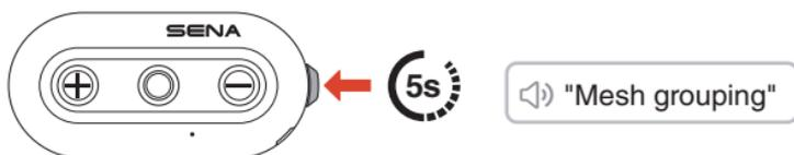
2. When mesh grouping is completed, it automatically switches from open mesh to group mesh.
